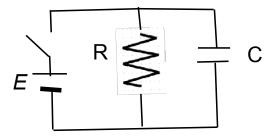
At t = 0, capacitor is fully charged by battery:  $\mathcal{E} = V_0 = Q_0/C$ . The battery is disconnected at t = 0. We use the loop rule for times t > 0:
